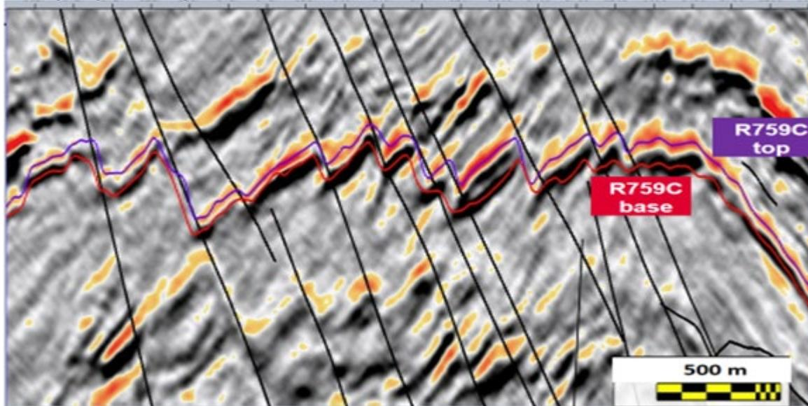
Figure 4. Zoom of structure at reservoir level for the far offset stack ( $30 - 42^\circ$ ). The interpretations in purple and red denote the top and base of the reservoir unit, respectively.
