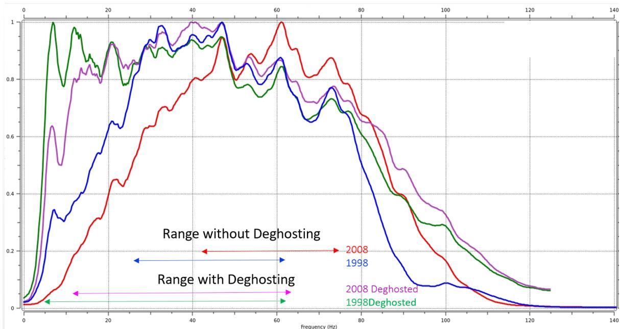
Figure 1: Extension of Spectra – with Deghosting
