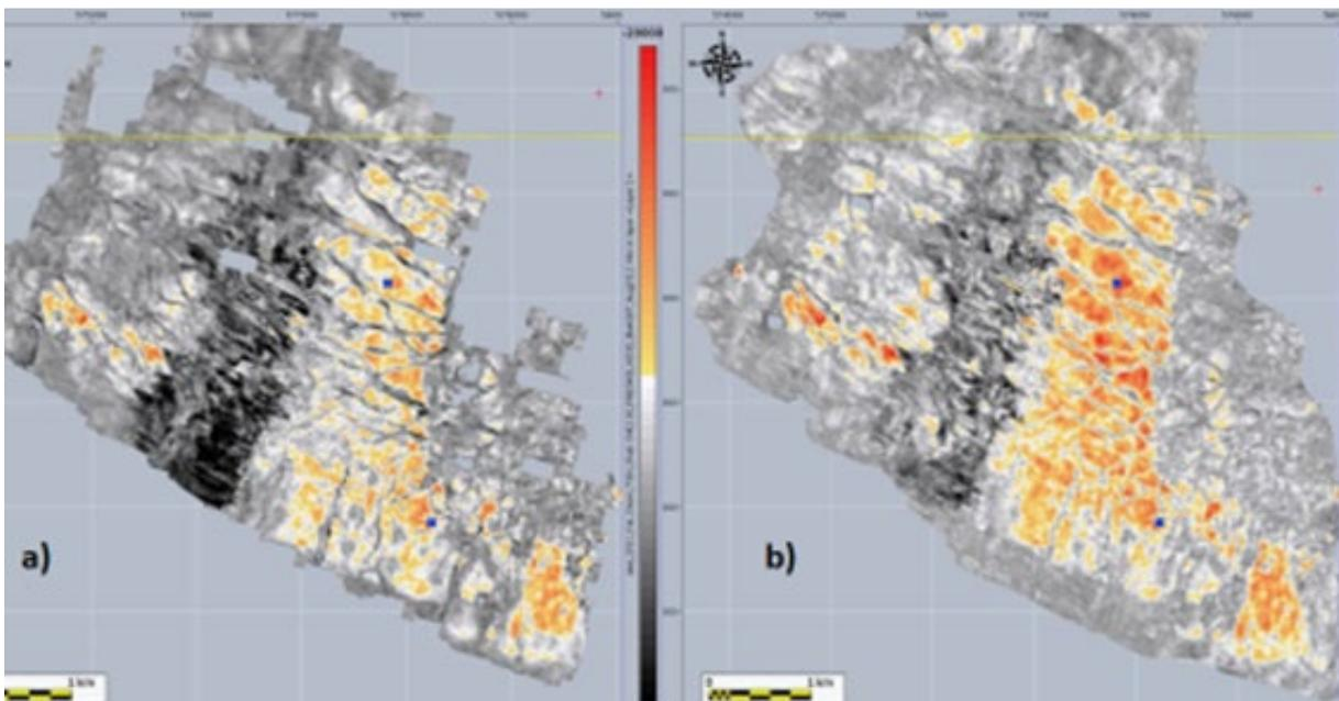
Figure 5. Amplitude map at reservoir level for far offset stacks ( $30 - 42^\circ$ ) for the minimum amplitude, for the 2011 results (a) and the new 2018 results (b). The new 2018 processing shows a much more coherent amplitude response, well bounded by faults.
