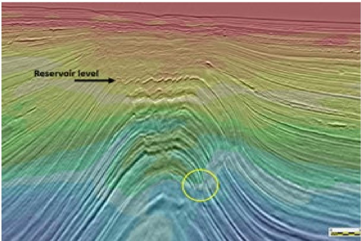
Figure 3. Kirchhoff preSDM images with model overlay for the 2018 results. Improvements are clear throughout the section, especially in the deep section where faults are clearly defined (e.g. yellow circle). The depth of the one of the reservoirs is indicated.
