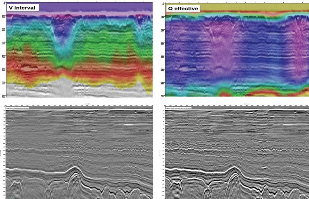
Figure 1. Top left: shallow section from a tomographic velocity model of North Sea broadband data. Top right: Q tomography highlights low Q (high attenuation) zones that need to be accounted for to optimize target resolution. Bottom left: broadband 200 Hz conventional Kirchhoff preSDM; Bottom right visco-acoustic (Q) preSDM (data courtesy of Polarcus).
