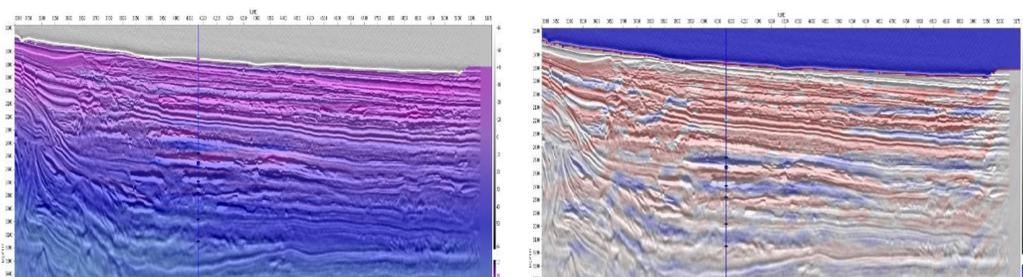
Figure 2. Deep water example, offshore West Africa. Left: smooth initial Q model. Right FWI Q inversion update, showing Q difference from initial model. The reservoir is clearly visible as a blue layer (with Q ~ 20) about halfway down the section around the well location, denoted by the vertical line (data courtesy of Ophir Energy).
