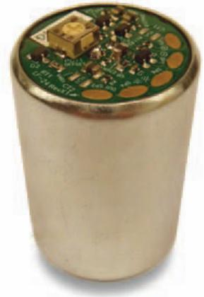
The LF-24/DC (Dual Compartment) Low Frequency Geophone has been designed to accommodate applications where the smallest form factor is required for vibration-monitoring and low-frequency seismic measurements. The device uses a low power electronic circuit to provide an inverse-filter function below the geophone natural frequency to compensate for the 12 dB/oct signal roll-off, extending the recording bandwidth.
