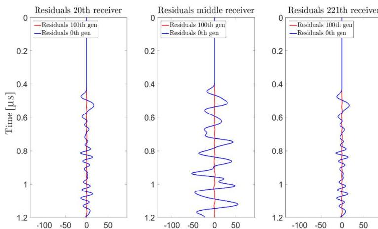
**Figure 3** The residual data related to the 20<sup>th</sup>, 120<sup>th</sup>, and 221<sup>th</sup> trace (from Figure 1b) of the worst model in the first generation (blue) and the best model in the 100<sup>th</sup> generation (red). The amplitude of the blue line is the same order of magnitude of observed data (Figure 1b).
