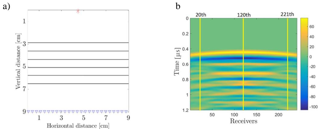
**Figure 1** a) Synthetic square sample with 6 horizontal fractures used in the experiment. Red star indicates the source location and blue triangles the receivers' locations. b) Observed velocity data modelled using the properties defined in the text for the sample in a). The yellow lines are the traces used to compute the residuals in the Figure 3.
