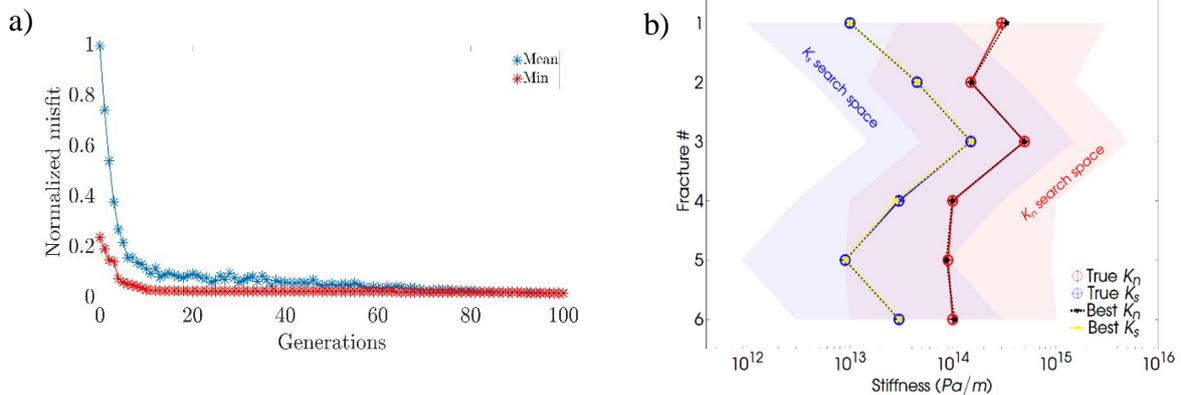
**Figure 2** a) The evolution of the normalized data misfit. b) Graphical representation of the comparison between the True and the Best model parameters of fractures. The shaded areas are the search spaces for  $K_n$  (red) and  $K_s$  (blue).
