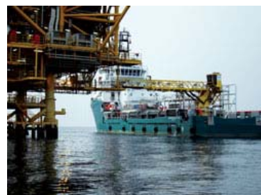
The Offshore Solution OAS is the only one of its kind to automatically compensate for the six movement planes of the vessel motion.
