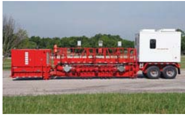
The CleanStream service unit enables effectively using ultraviolet light to control bacteria in fracturing fluids.
