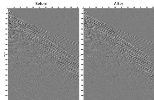
Figure 10: Example of SI attenuation in Tau-P domain on common shot gathers (negative dips/interference from astern)
