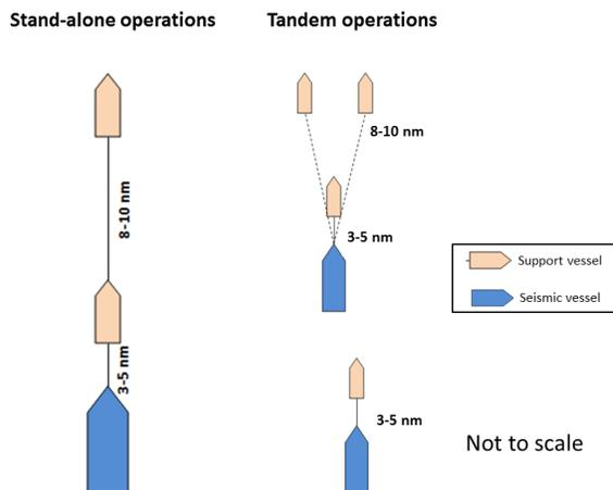
Figure 4: Optimal ice management vessel positions
