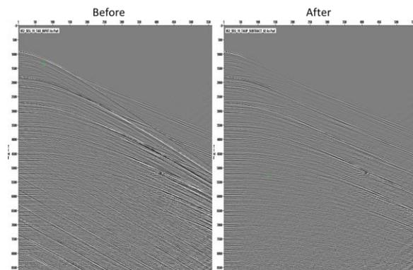
Figure 9: Example of SI attenuation in Tau-P domain on common shot gathers (positive dips/interference from ahead)
