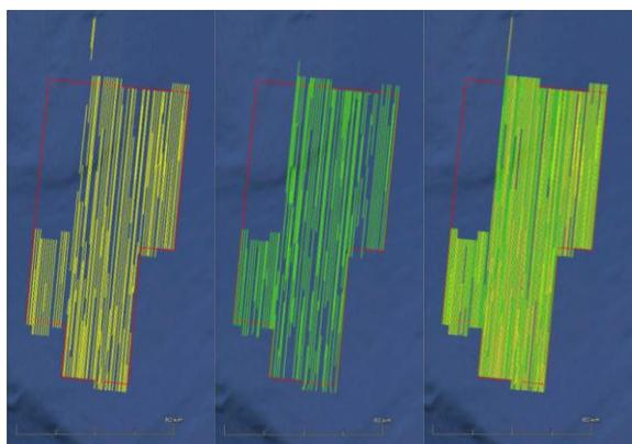
Figure 6: Final post-plot maps showing prime and infill lines acquired by individual vessels on the left and combined survey on the right
