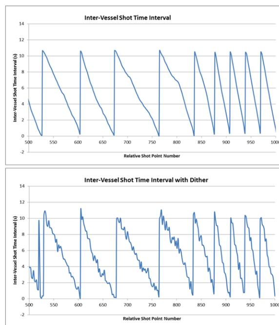
Figure 7: Inter-vessel shot time interval without (top) and with (bottom) application of source dither
