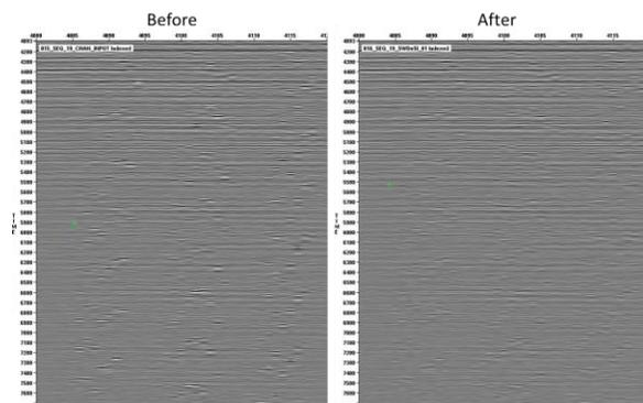
Figure 8: Example of SI attenuation after random-noise attenuation application on common channel gathers
