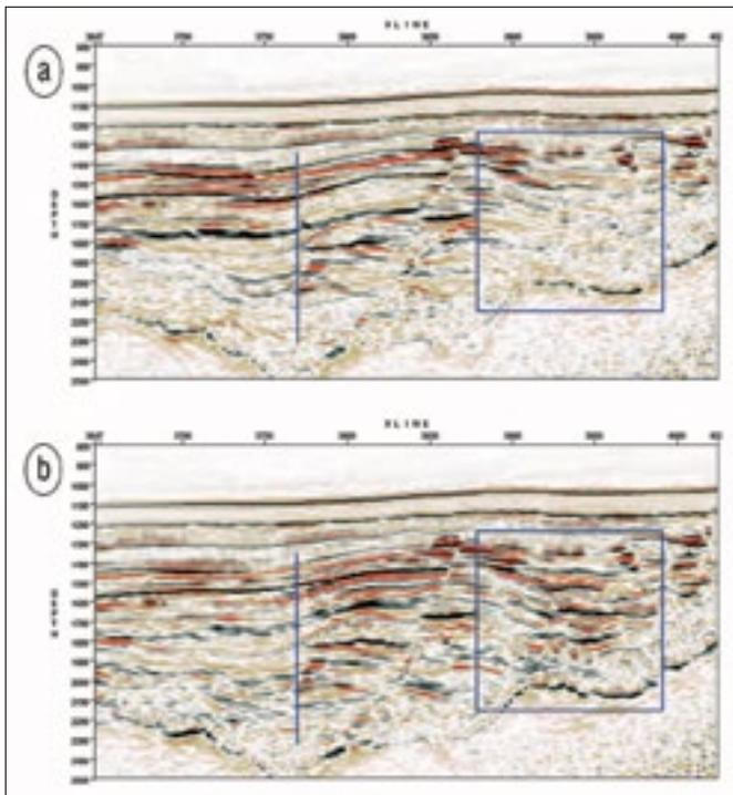
**Figure 3.** (a) Stack image using the initial velocity model and the initial epsilon model before anisotropic WFI. (b) Stack image using the updated velocity model and the updated epsilon model after anisotropic WFI.
