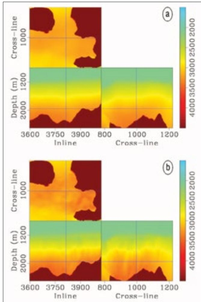
**Figure 4.** (a) Initial velocity model before visco-acoustic WFI. (b) Updated velocity model after visco-acoustic WFI. Upper left = depth slice, lower left = inline slice, lower right = crossline slice.
