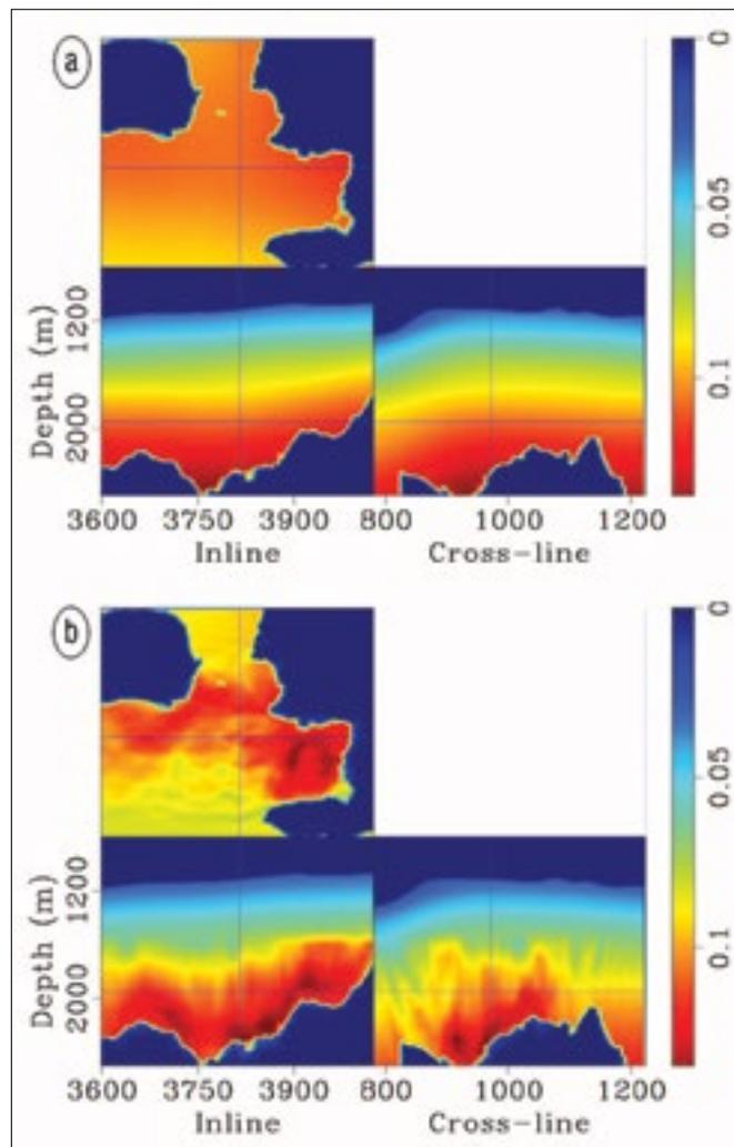
**Figure 2.** (a) Initial epsilon model before anisotropic WFI. (b) Updated epsilon model after anisotropic WFI. Upper left = depth slice, lower left = inline slice, lower right = crossline slice.
