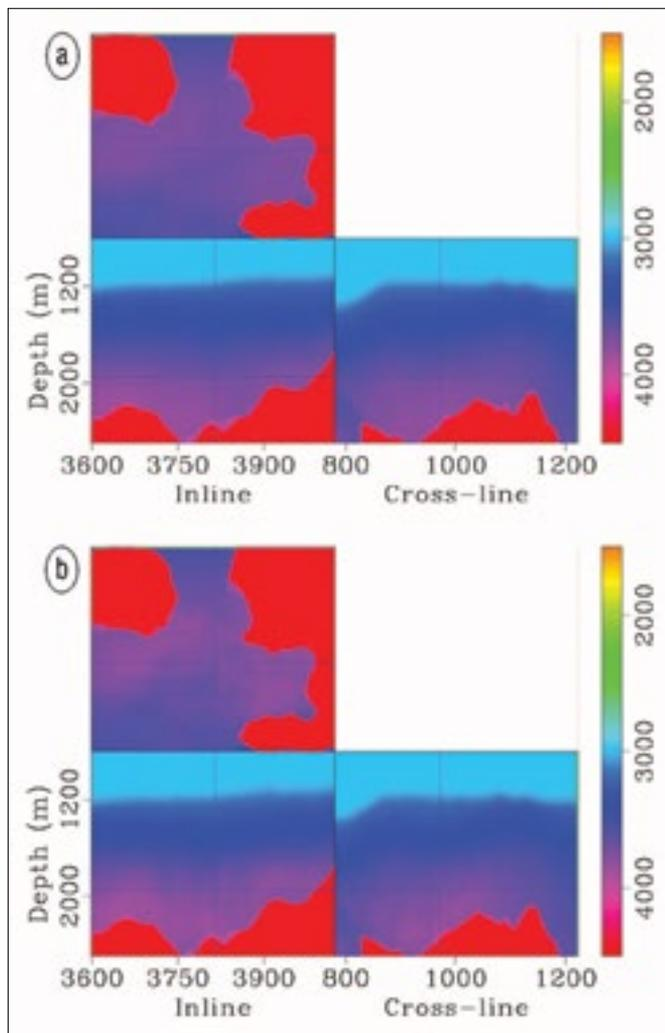
**Figure 1.** (a) Initial velocity model before anisotropic WFI. (b) Updated velocity model after anisotropic WFI. Upper left = depth slice, lower left = inline slice, lower right = crossline slice.
