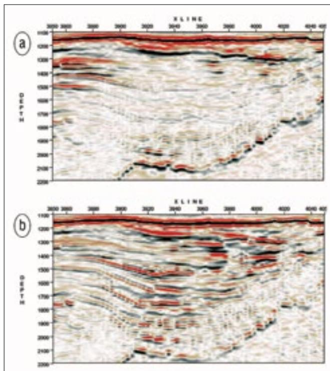
Figure 6. (a) Initial stack image before visco-acoustic WFI. (b) Updated stack image after visco-acoustic WFI.
