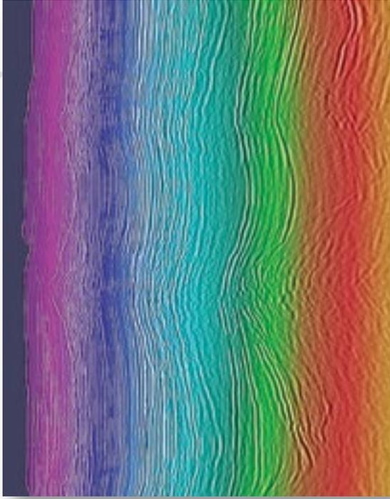
*Velocity model before application of general moveout tomography.*
