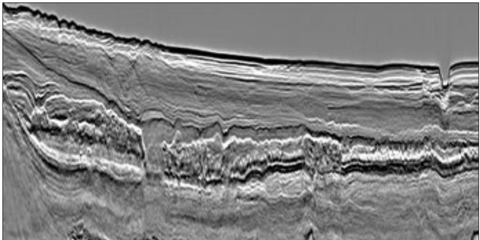
**Figure 10.** Same data as in Figure 9, imaged after WiBand deghosting. A 160-Hz high-cut filter is applied.
