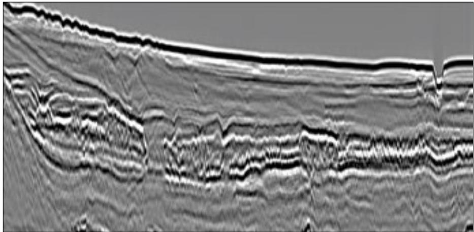
**Figure 9.** PSTM image of NE Greenland SPAN data without deghosting. Source is at 18 m depth below sea surface, and streamer is at 20 m depth. A 55 Hz high-cut filtered is applied. Vertical axis is two-way time in seconds. Horizontal axis is distance divided by 6.25 m.
