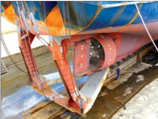
**Figure 8.** The skag for enabling subsea streamer deployment.
