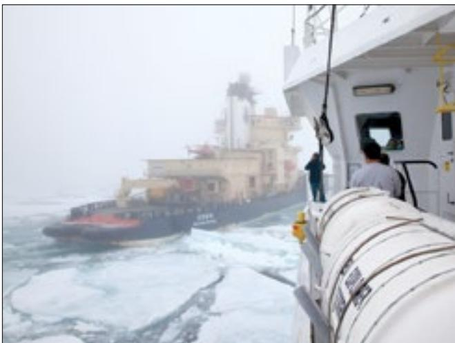
*Figure 4. Icebreaker Oden operating in close escort with seismic vessel during acquisition.*
