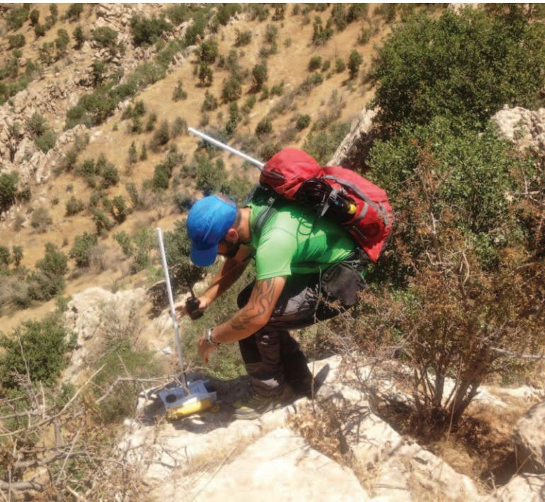
A worker deploys an RT System 2 wireless remote unit in the rugged terrain of Kurdistan. (Source: Wireless Seismic)
