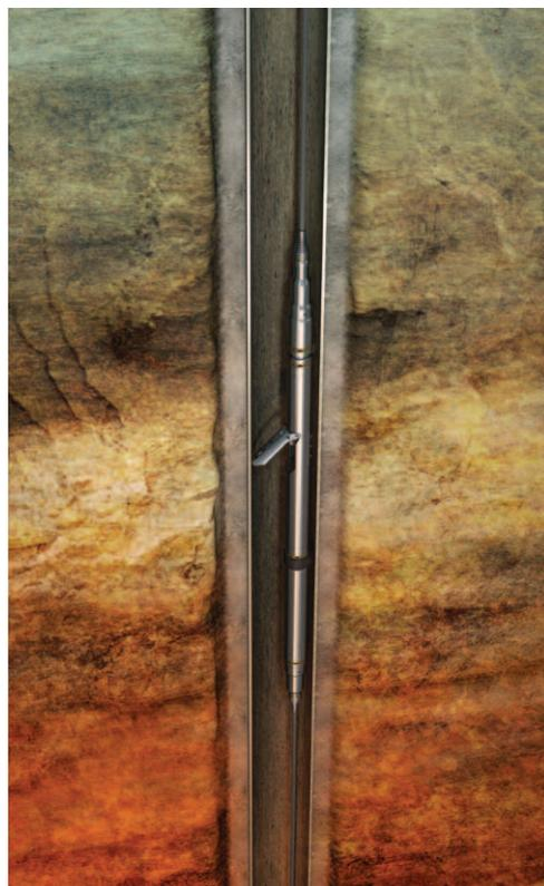
**The GeoWave II downhole seismic tool can conduct safe and efficient VSP and hydraulic fracture monitoring surveys in the most hostile well environments. (Source: Sercel)**
