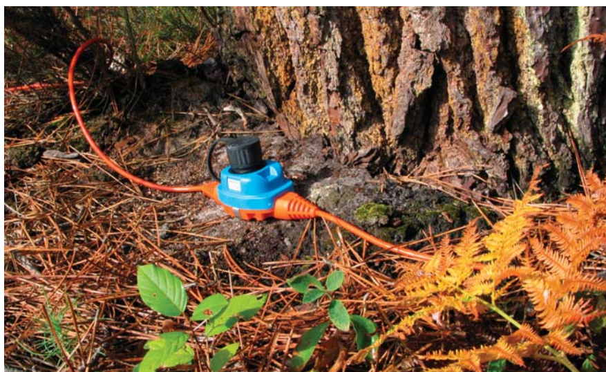
Sercel's fifth-generation digital recording system is designed to accommodate high channel counts and greater layout flexibility in either a single-component or multicomponent configuration. With a capacity of 100,000 channels, the system provides accuracy, speed and ease of use in even the largest survey.
