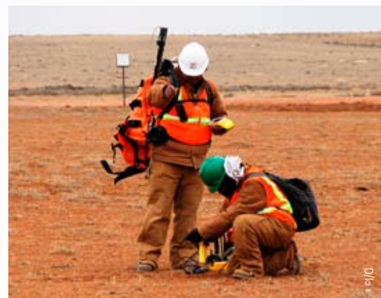
Cableless systems can be used with smaller crews carrying lightweight backpacks, enabling deployment around steep terrain and obstacles in the field.
