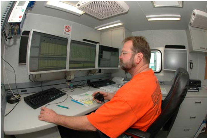
Typical central electronics configuration in recording truck.
