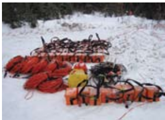
ARIES is a cable-based seismic recording system designed for use in all environments
