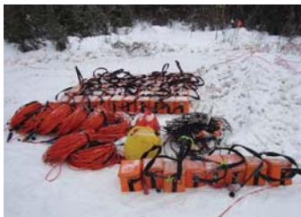
ARIES is a cable-based seismic recording system designed for use in all environments.
