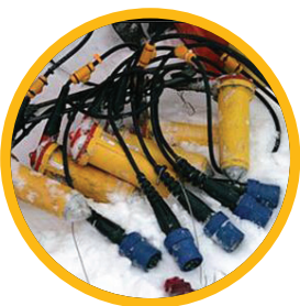
VectorSeis receivers being prepared for deployment.
