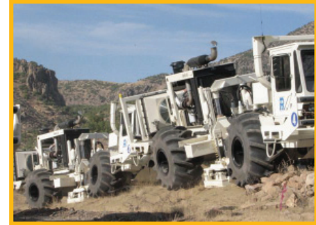
ION's AHV-IV vibrators were recently commissioned and utilized with Pelton Vib Pro controllers.
