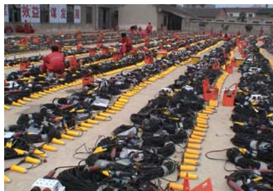
VectorSeis sensors and the land acquisition system being prepared for deployment.
