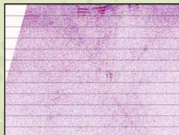
Stack after interference noise attenuation
