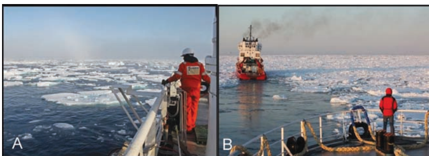
Figure 3 Ice conditions during acquisition – 3a: June 2010 coverage, 3b: September 2010 coverage. Note icebreaker leads the acquisition ship to clear a path through first-year ice.
